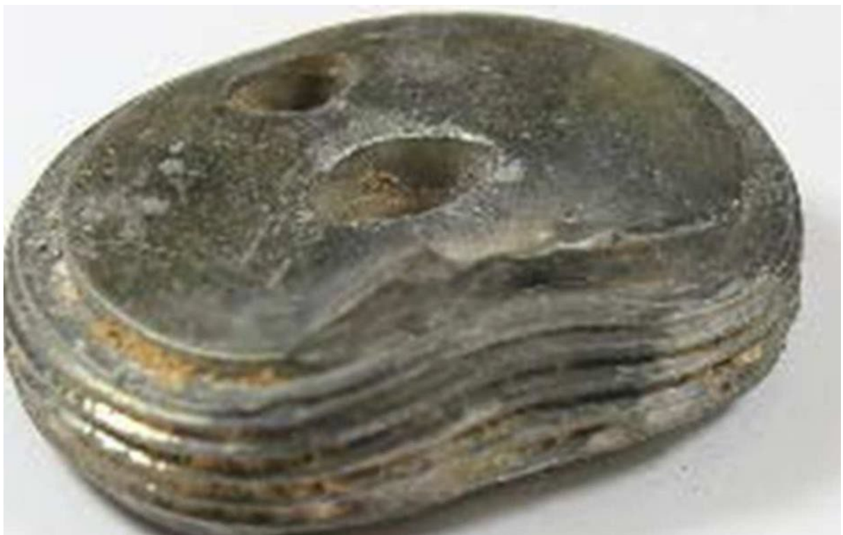
Figure 10: Enlargement of the cover plate shows possible presence of sand in the thread. (Picture: TNO)
