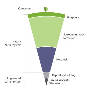
The relative contributions to safety of the various barriers at different times after closure of a disposal facility and the ways that they interact with each other depend upon the design of the disposal system. The design itself is dependent on the geological environment in which the facility is constructed. Consequently, the multibarrier system can function in different ways at different times in different disposal concepts.
