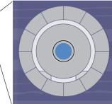
The disposal tunnel has a concrete liner for mechnical support. After emplacement of the supercontainer in the tunnels. the void space between the container and the lines are backfilled with foamed concrete.
