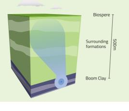
The lithostatic load of the geological formations overlying the tunnels will be taken up by the tunnel liner. The concrete is expected to degrade slowly by reaction with clay pore waters, inwards from the Boom Clay / tunnel liner interface. Since the degradation will penetrate only a few tens of millimetres into the liner after 1000 years, it is unlikely that this very limited decalcification could cause the liner to begin to lose compressive strength.
