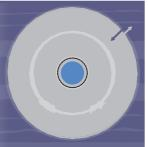
Concrete components of the EBS undergo slow mineral transformation controlled by diffusion from and into the Boom Clav. slow diffusion-dominated, anoxid corrosion of the overpack continues. Most of short-lived radioactivity has decayed in-situ.
