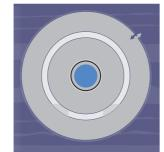
Pore water very slowly diffuses into concrete liner and cement components diffuse into clay. Slow diffusion-dominated, anoxic corrosion of the overpack has started. RRSF has cooled down, but has not come into contact with water.
