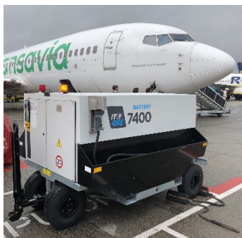
eGPU supplies power to stationary aircraft without emissions
