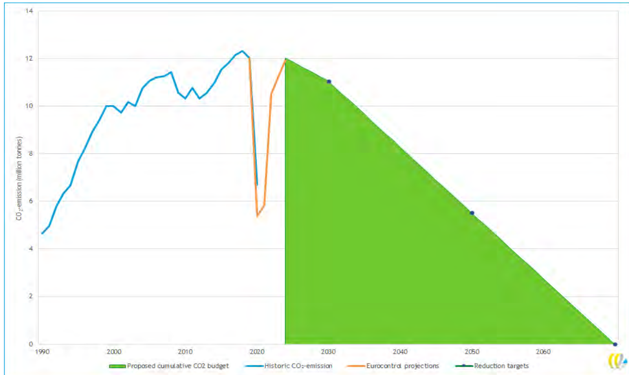
Figure 1 - CO 2 -emissions on the basis of tanked kerosine in the Netherlands 11 ; the proposed cumulative CO 2 budget is shown in green
