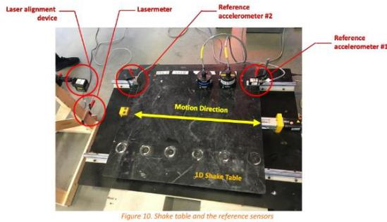
Figure 10. Shake table and the reference sensors
