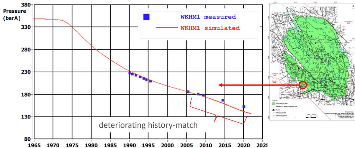
Starting point of the calibration is the new version of dynamic reservoir model version 7, that incorporates several corrections and updates in both the static and dynamic part of the model compared to version 6 (ref. 46 to 48).
