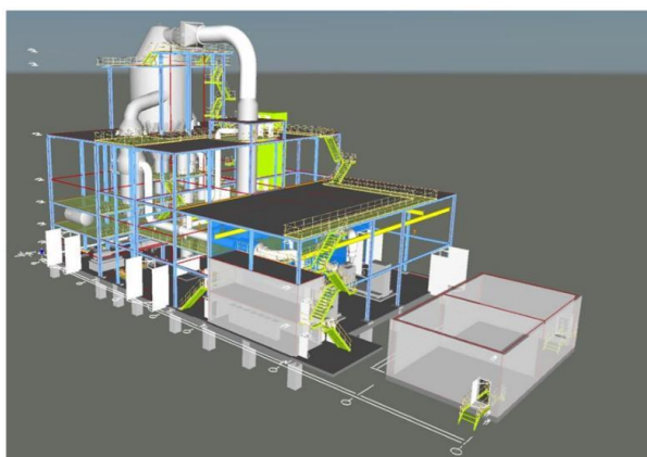
Figure IV.2: 3D model of a single 700 kt MVR unit. Typical footprint: 32m wide, 61m long and 33m high.
