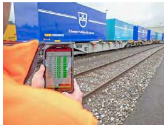
An automatic brake test.
