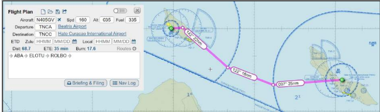
Figure 12 - Aruba to Curaçao Planning Chart Example
